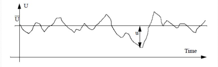
The velocity is divided into an average value U, and a fluctuating value u. The two variables are inserted into the Navier-Stokes equation for laminar flow, and after some manipulations and simplification the Navier-Stokes equation for turbulent flow emerges:
