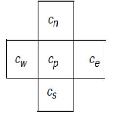
$a_e$ : weighting factor for *cell* e $a_W$ : weighting factor for *cell* w $a_n$ : weighting factor for *cell* n $a_s$ : weighting factor for *cell* s $a_p = a_e + a_W + a_n + a_s$
