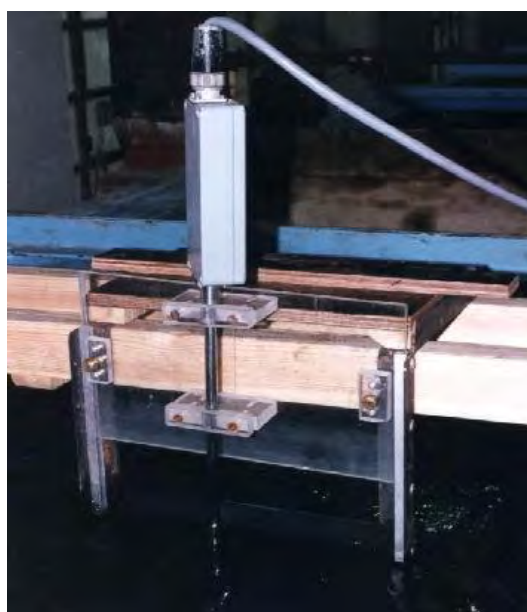
Photo 3-4: The electromagnetic currentmeter
