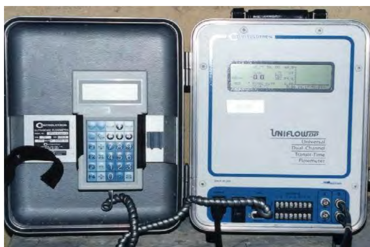
Photo 3-3: The ultrasonic flowmeter
