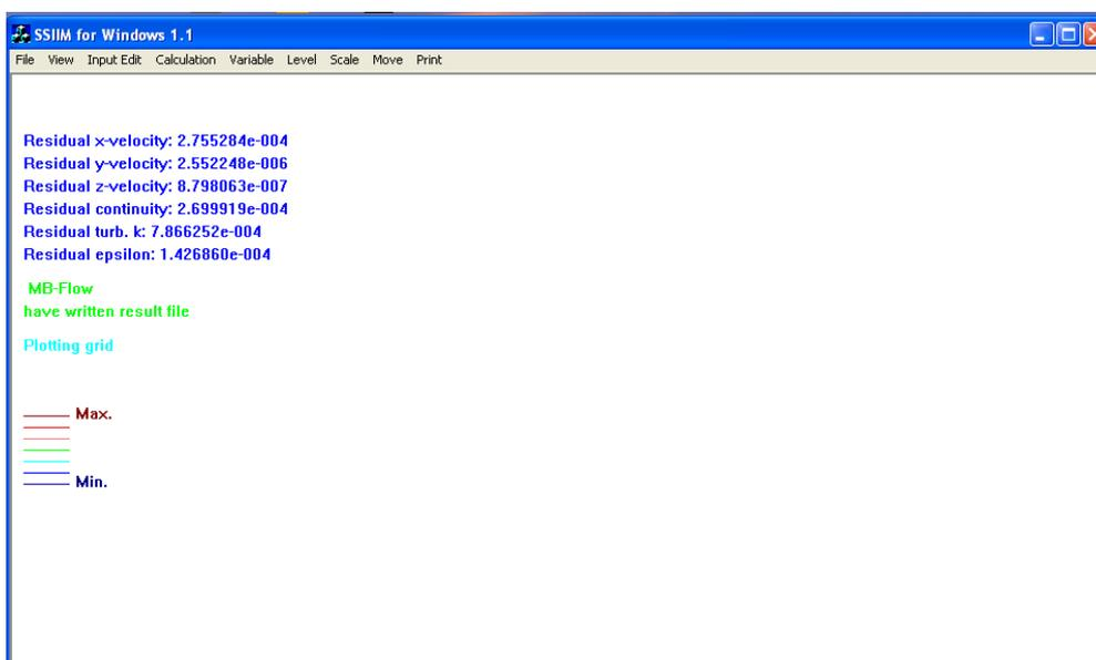
**Figure 3-1:** Text window of the SSIIM program showing the residuals for the iterative calculations of the six parameters
