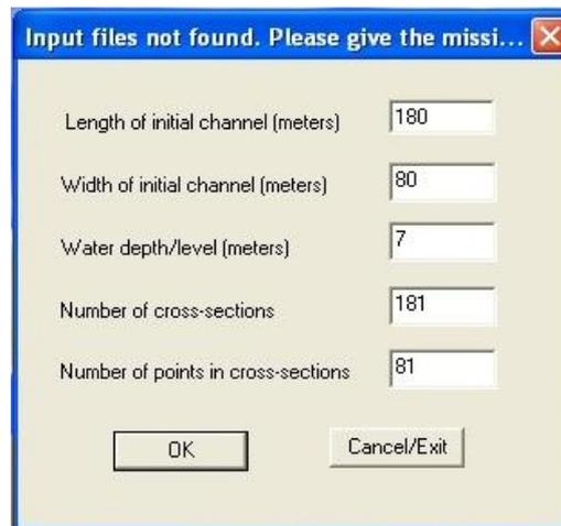
**Figure 3-2:** SSIIM Dialog Window for setting the initial parameters of the structure
