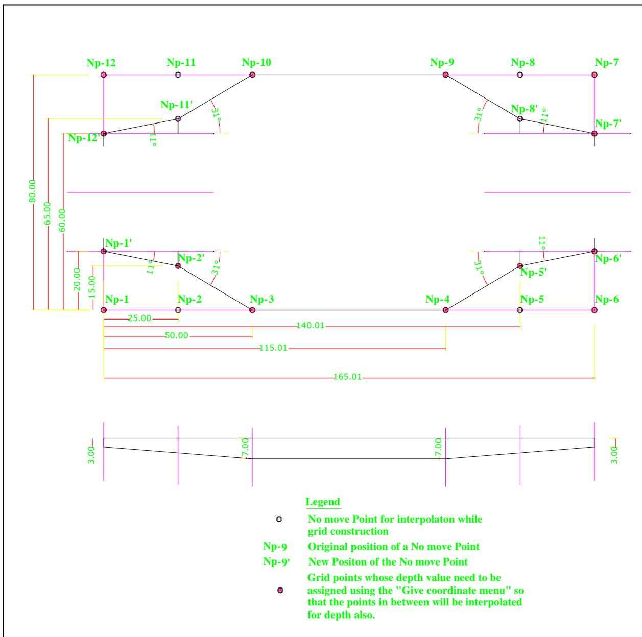
**Figure 4-1:** Design including the transition zone to be modeled numerically using the SSIIM program
