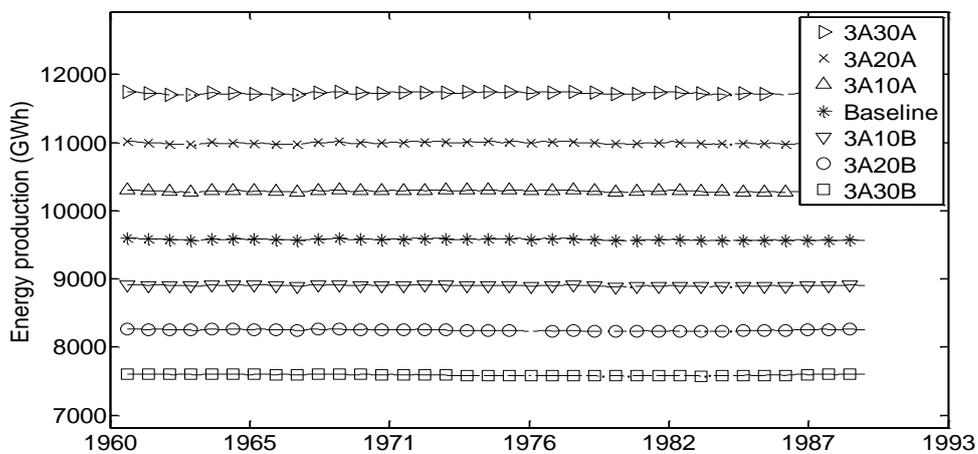
**Figure 6.6 :** Energy production variation for different climate scenarios with a temperature increase of 3°C at Giteranyi
