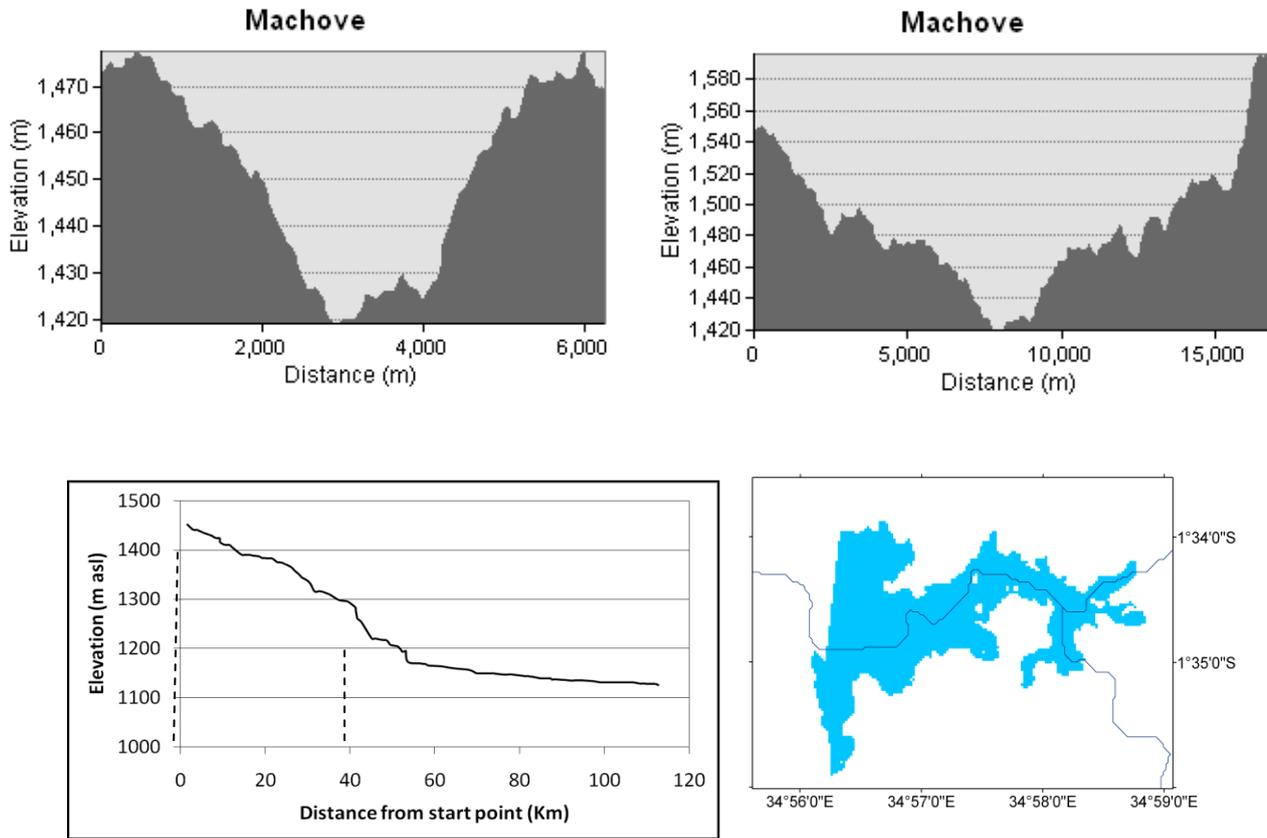
**Figure 4.7:** Details for the selected hydropower site at Kilgoris including (a) Dam physiology, (b) Dam Vicinity (c) location at Reach 1 and (d) the reservoir extent.
