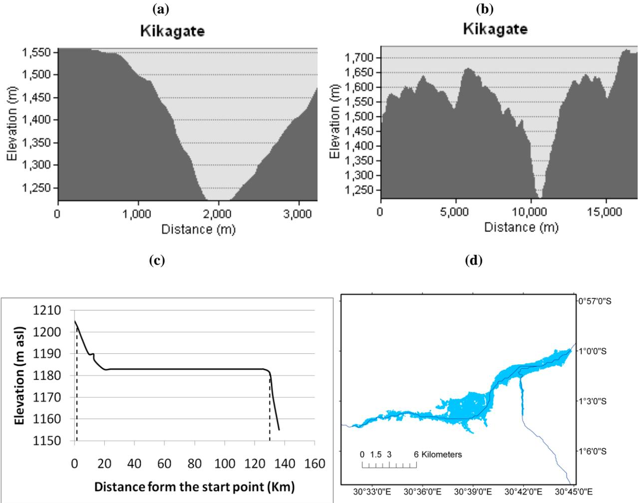
**Figure 4.4:** Details for the selected hydropower site at Kikagate including (a) Dam physiology, (b) Dam Vicinity (c) location at Reach 4 and (d) the reservoir extent.
