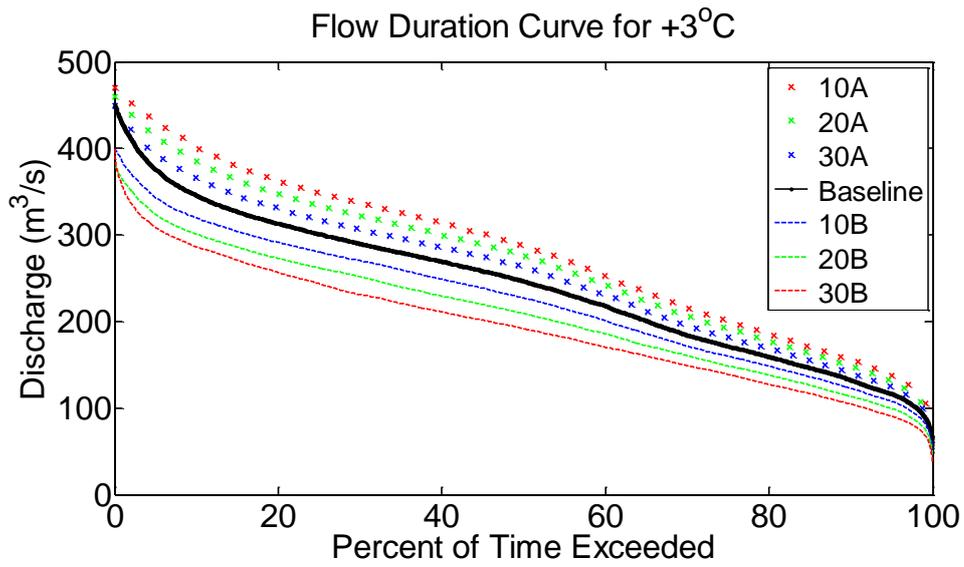
Figure 5.2 : Flow Duration Curve for Giteranyi
