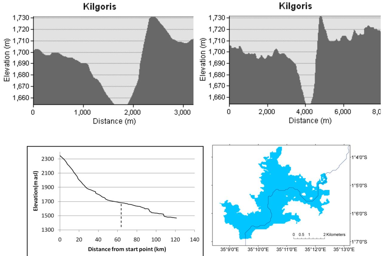
**Figure 4.6:** Details for the selected hydropower site at Kilgoris including (a) Dam physiology, (b) Dam Vicinity (c) location at Reach 3 and (d) the reservoir extent.
