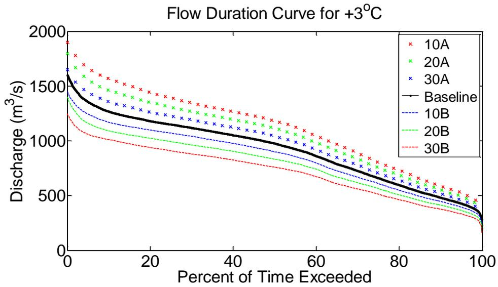
Figure 5.6: Flow Duration Curve for Kikagate
