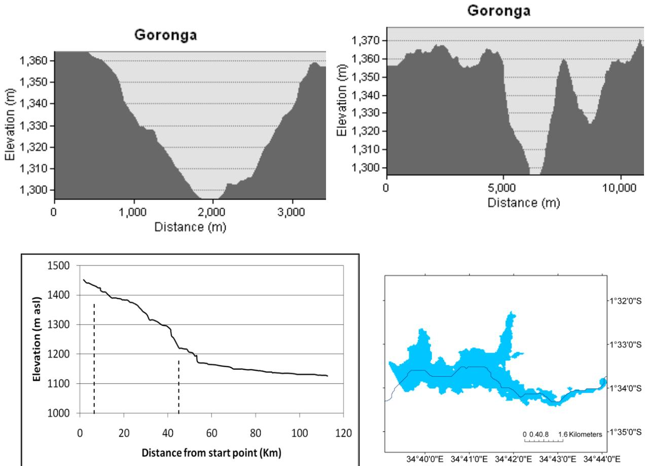
**Figure 4.8:** Details for the selected hydropower site at Goronga including (a) Dam physiology, (b) Dam Vicinity (c) location at Reach 1 and (d) the reservoir extent.
