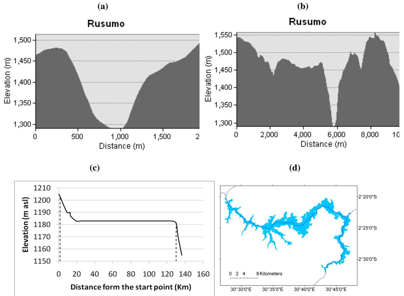
**Figure 4.3:** Details for the selected hydropower site at Rusumo including (a) Dam physiology, (b) Dam Vicinity(c) Location at reach 4 and (d) the reservoir extent.
