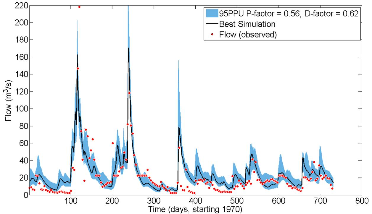
**Figure 3.13:** Calibration results for Mara mines station in Mara catchment
