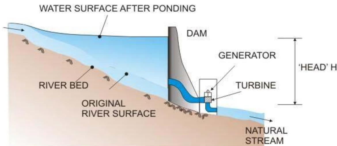
**Figure 6.1:** Set up of a Dam
