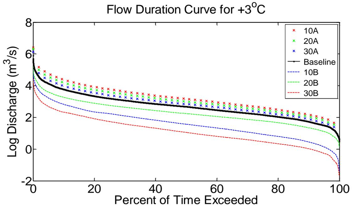
Figure 5.10: Flow Duration Curve for Machove +3°C
