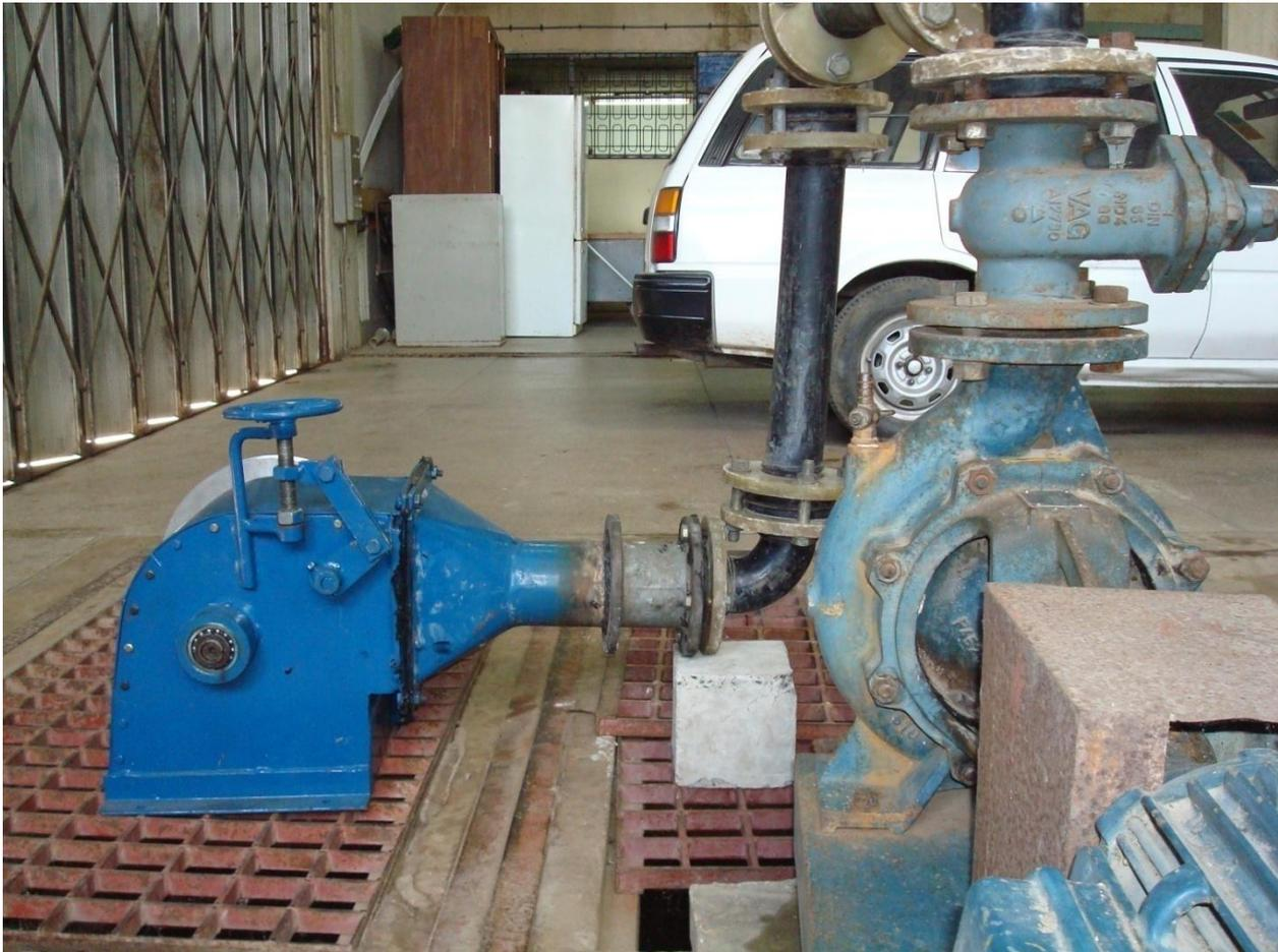
**Figure 4. 1 Cross flow turbine testing (Wakati (2010))**
