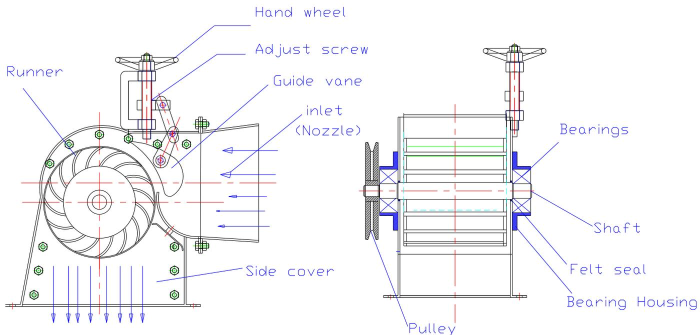
**Figure 3.2 Detail of the locally designed cross flow hydro turbine**
