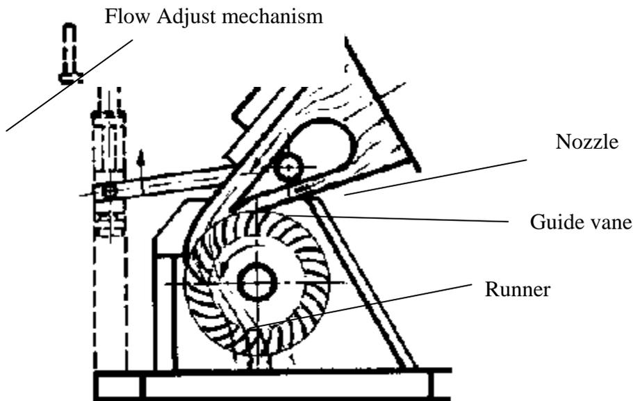
**Figure 3.1: Schematic diagram of Cross flow Turbine (adopted from Wakati, 2010)**
