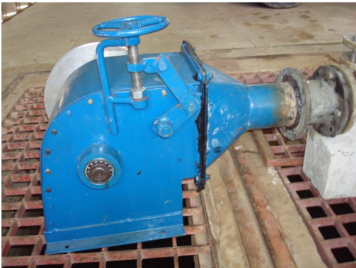
**Figure 3.4** Turbine casing and finishes
