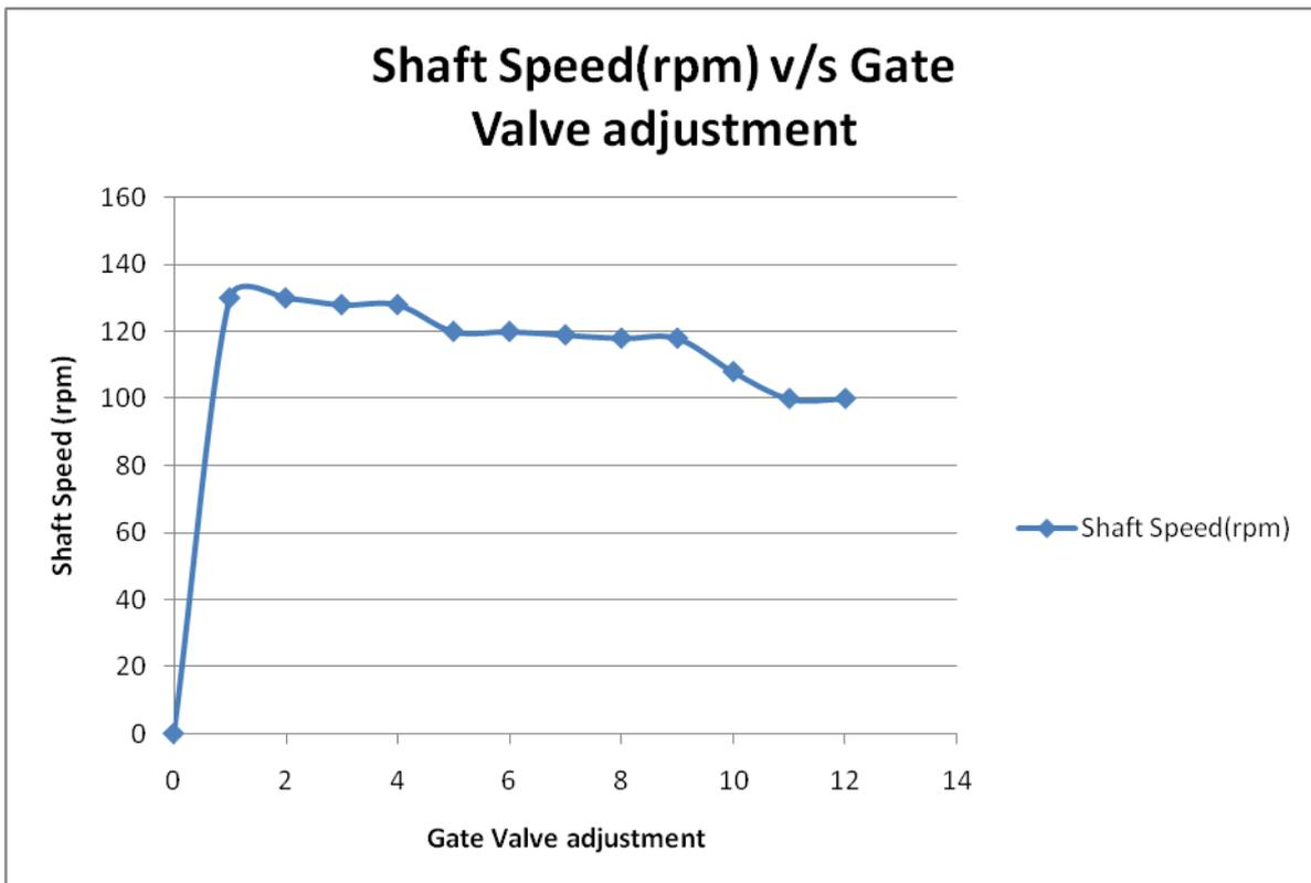
Figure 4.2 Shaft speed versus valve adjustment (Wakati (2010))
