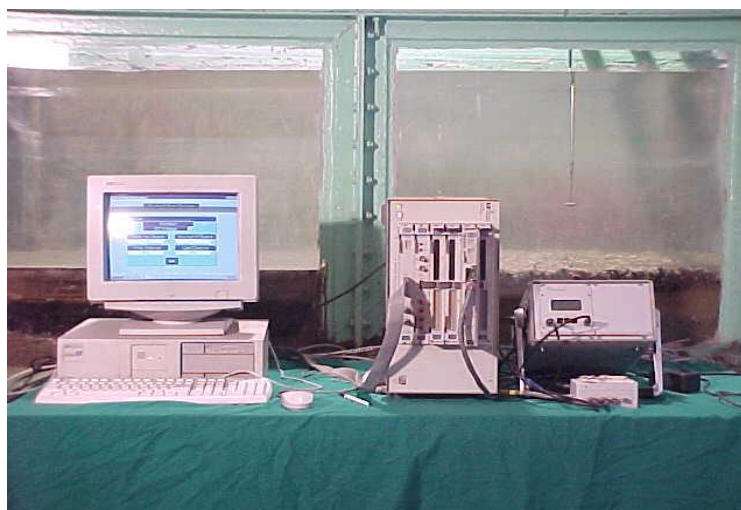
Photo 3-7: Data Acquisition systems and the data logger
