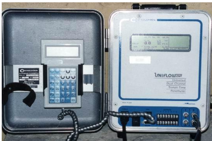
Photo 3-3: The ultrasonic flowmeter
